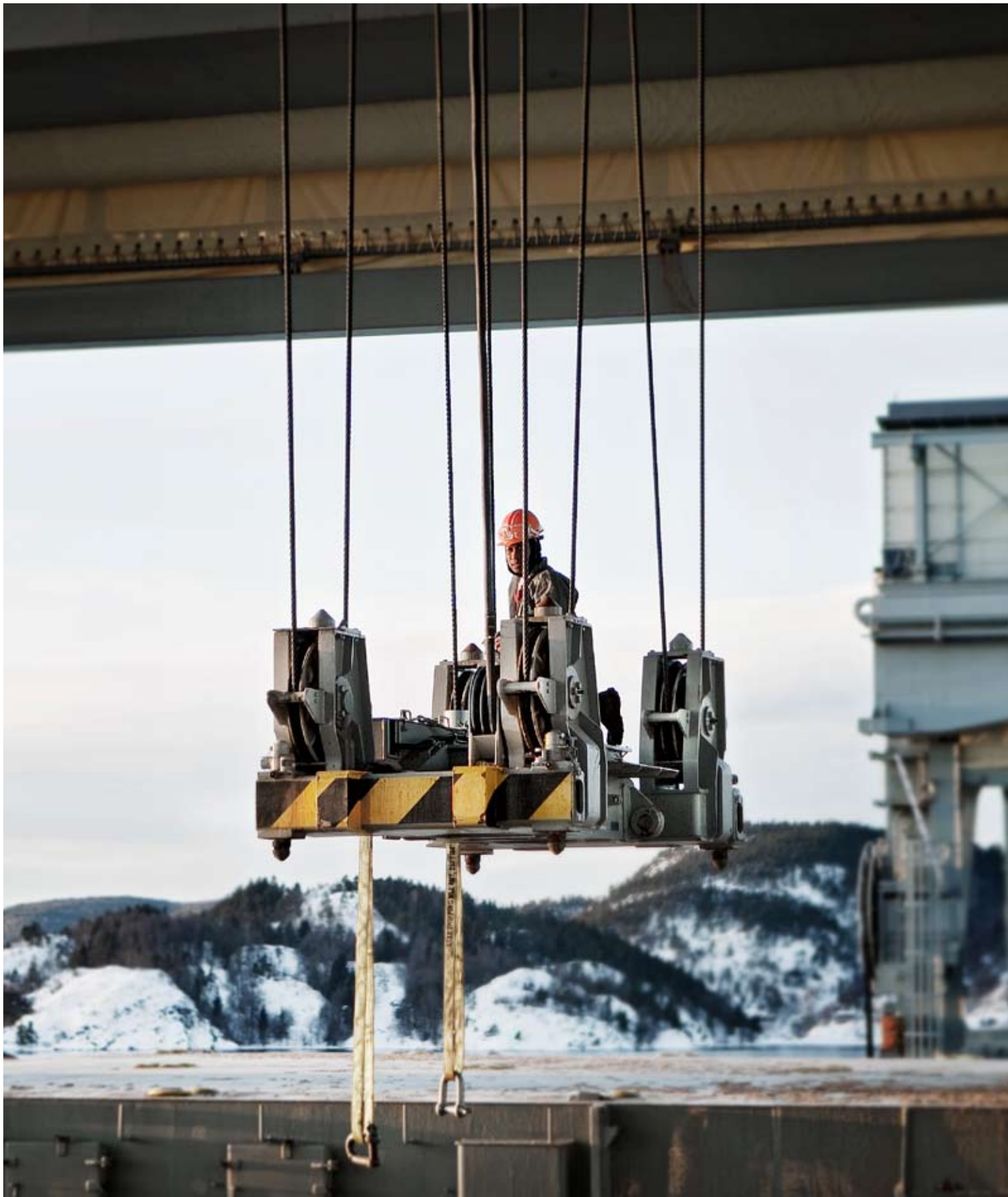
Preparing to unload cargo from the open hatch hold. The onboard gantry cranes on the K class vessels can lift 70 tons each.
