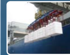
60 ton lift of pulp being loaded using Grieg Star Shipping's unihooks.
